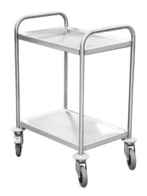
The Stainless Steel Cleanroom Trolley uses high-quality 304-grade stainless steel to deliver both durability and easy maintenance. It includes two shelves, each supporting up to 40 kg, making it ideal for transporting equipment in environments that demand hygiene and sturdiness. The trolley measures  $895 \times 595 \times 950$ mm in overall, and each shelf is  $800 \times 500$ mm. A 590mm gap between the shelves provides ample space for a variety of items.
